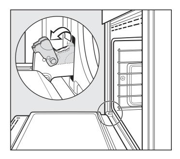
■ Slowly shut the door until the protruding clamps stop the movement. Pull the door upward. See illustration.
